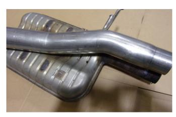
Remove the original system, place the resonator delete pipe over the top of the system.
